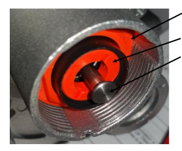
OPSO (overpressure shut off )adjustment under orange cap outside orange ring adjust with tool. Clockwise for increase.
