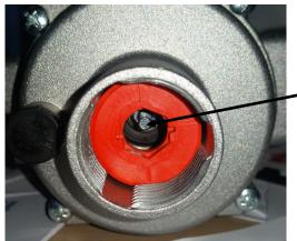
Main Pressure adjustment (under black cap) use tool on orange disk. Clockwise for more pressure. Anticlockwise for less.
